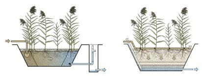
Figure 2 Overview schematics of HSSF (left) and VF (right) CW (Dotro et al. 2017).
