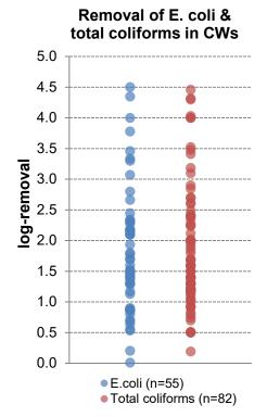
Figure 5 Log-removal of *E. coli* (blue dots) and TC (red dots) in literature data.
