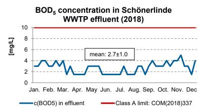
Figure 28 BOD₅ concentration in the effluent of Schönerlinde WWTP in comparison to the class one limit of the proposed EU-level water reuse regulation (COM337, 2018).
