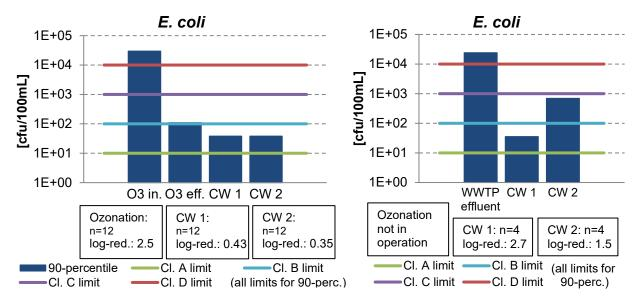
Figure 29 Concentration of E. coli (in the relevant percentile) during ozonation and treatment in two parallel CWs, with relevant limits of COM337 (2018). Log-red: log reduction, Cl.: class.
