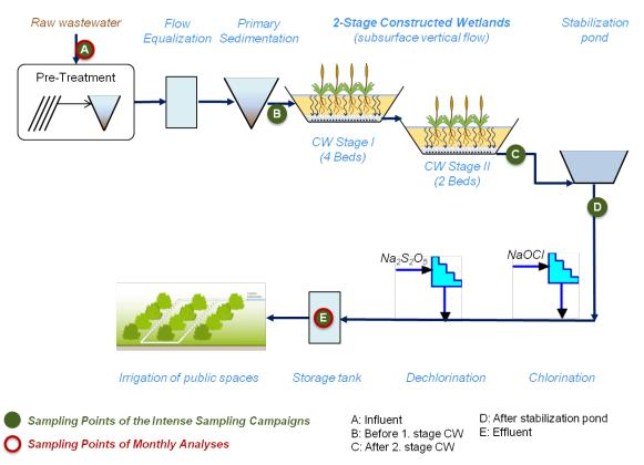
Figure 8 Flow scheme of the Antiparos WWTP including sampling points
