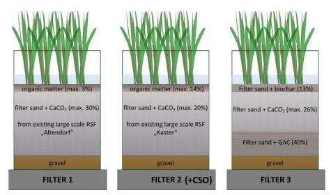
Figure 31 Schematic view of the three pilot RSF at at Rheinbach, Erftverband.
