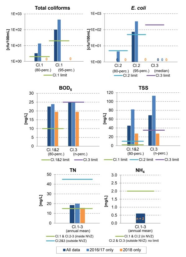
Figure 16 Compliance of relevant percentiles for all samples (dark blue), samples taken 20167/17 before reconstruction measures (light blue) and 2018 after reconstruction (orange) with limit values of the Greek water reuse regulation [NVZ: Nitrate vulnerable zones], for n-perc.-values see Table 13.
