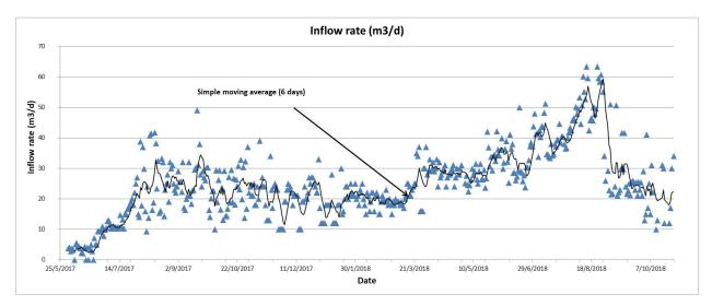
Figure 20 Inflow rate of wastewater into the Thirasia WWTP since the beginning of its operation.
