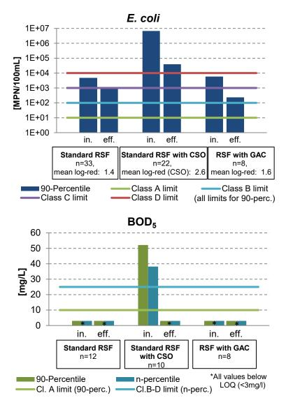
Figure 32 Concentrations of *E. coli* and BOD₅ in influent (in.) and effluent (eff.) of the three pilot RSF at Erftverband with associated limits of COM337.
